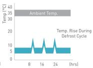
At 35°C, no load, measured at center of chamber.
